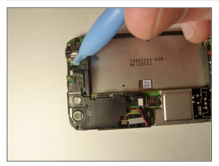
Pry off the camera lens using a plastic opening tool.
