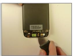
• Use a Jimmy to pry up the OEM SIM and SD card reader contact.
