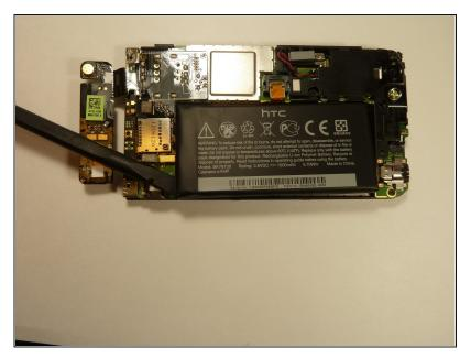
Pry up the battery with the flat end of the spudger.
