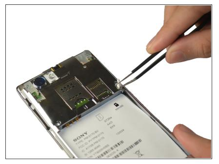
Remove the silicone cover by squeezing it with the tweezers, there is not much pressure needed.
