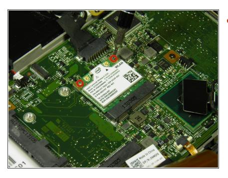
Remove the two silver 3mm screws with a Phillips 00 screwdriver.
