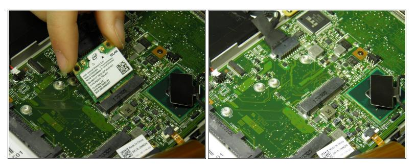
• Angle the wireless WLAN card upward and remove it.
