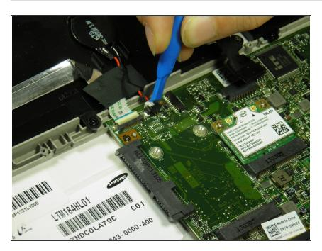
Use the plastic opening tool's angled edge to remove the red and black CMOS battery cable.
