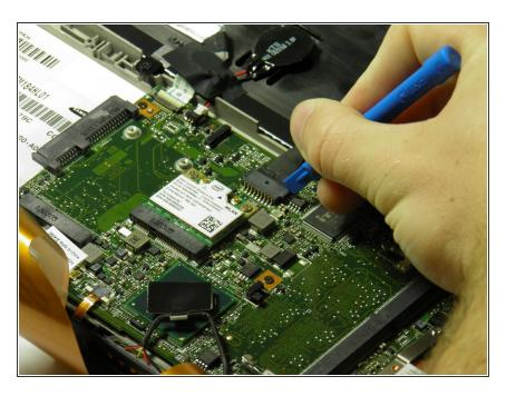
Use the plastic opening tool's angled edge to pry the black battery cable loose.
