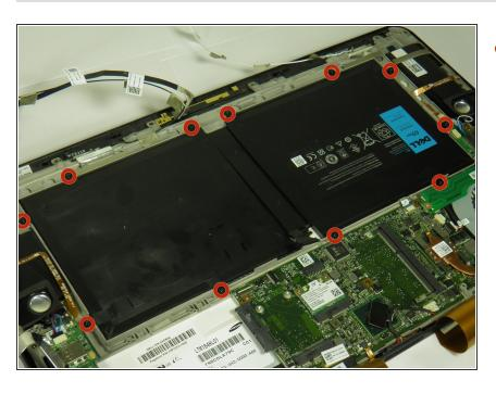
Remove the eleven black 4mm screws holding the battery in place with a Phillips 00 screwdriver.
