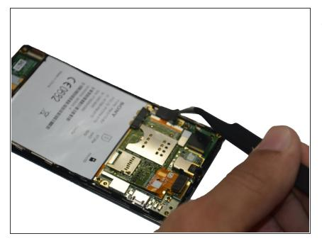
Then remove the sticky pad located at the left of the phone using he tweezers.
