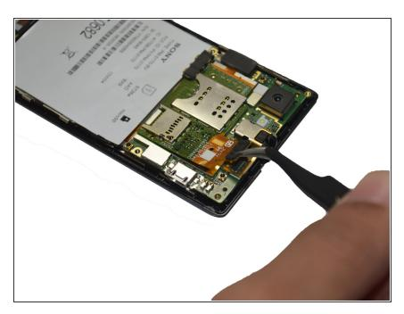
• Using the tweezers remove the clip located at the top of the phone. It should snap right off without too much pressure.
