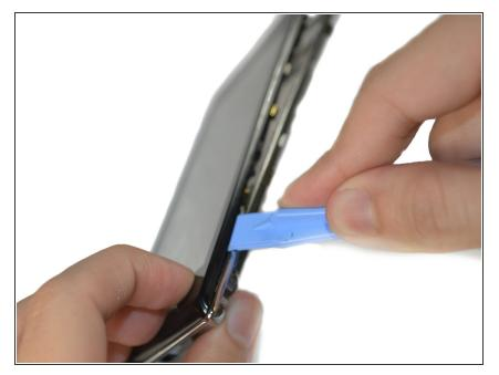
Place the plastic opening tool inbetween the black external case of the phone and the silver case, then move it along the edges of the phone to detach the plates.
