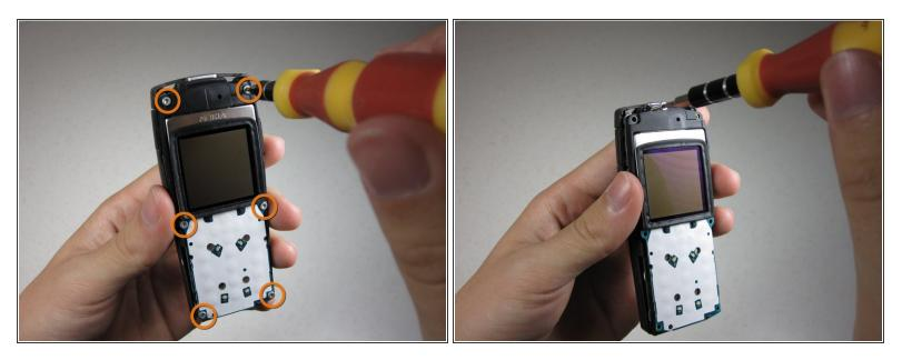
• Using a T6 Torx Screwdriver, unscrew and remove the six screws shown in the picture.
