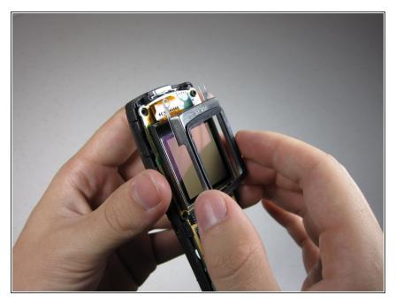
• Remove the LCD screen frame.
