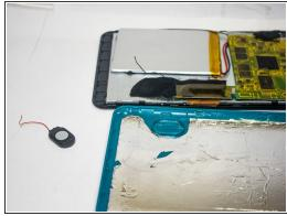
Remove the speakers by using your hand to entirely disconnect the back cover.
