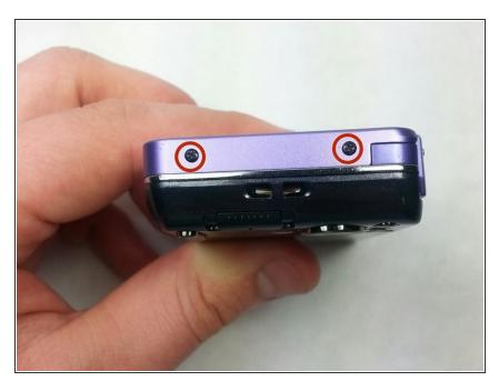
Turn the camera sideways so the left side is fasning upwards, remove the two Phillips head, 2.93 mm screws.
