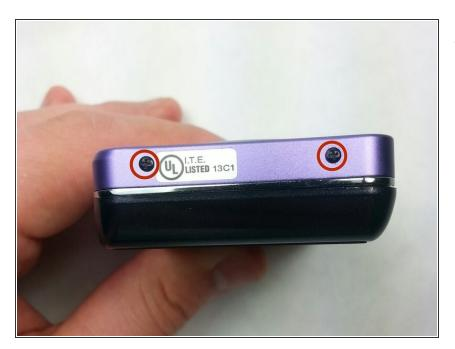
Now turn the device so the opposite side is fasning upwards and remove the last two Phillips head, 2.93 mm screws.
