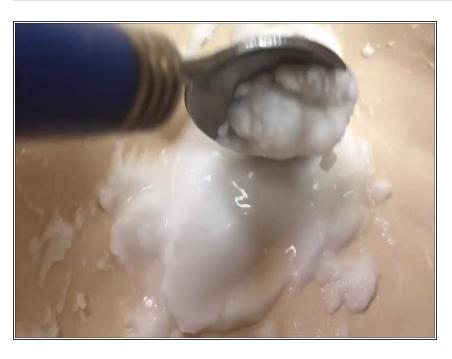
The consistency of the paste should be similar to a thick and grainy toothpaste.
