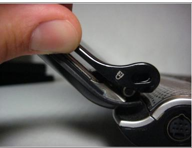
Press the tabs on the sides of the screen in and pop the plastic off. Careful, the plastic is very flimsy and may break.
