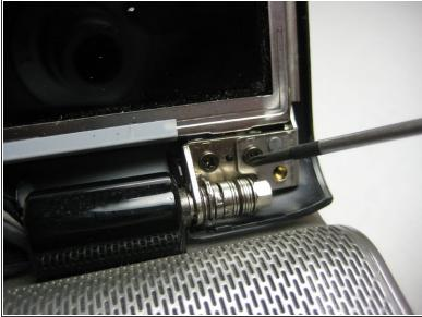
Remove the two screws (5.8mm) on either side of the LCD near the hinge. Remove the screws on the outermost side first.
