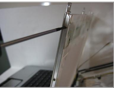
Take out the two 3.58mm screws on the LCD at the top (one on each edge).
