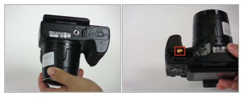
A Electric shock is a huge risk if the battery is not removed while taking the camera apart.
