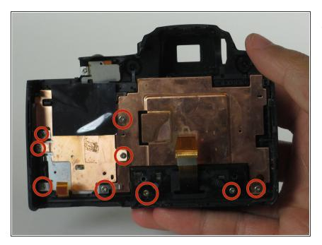
Remove the labeled 3mm screws using a PH00 screwdriver.
