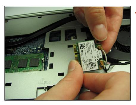
Disconnect the two antennas (one black and one white) from the wireless card.
