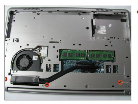
Unscrew the three black 5 mm screws with the Phillips head screwdriver.
