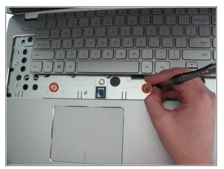
Unscrew the two black 5 mm screws underneath the keyboard using a Phillips head screwdriver.
