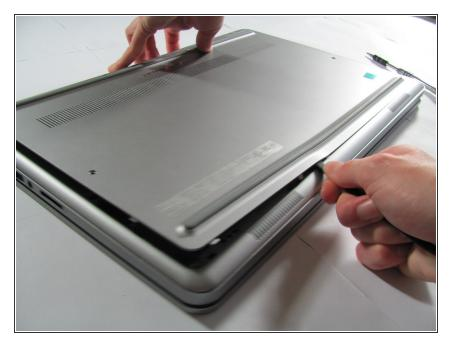
• Use a spudger to remove the base cover from the rest of bottom cover.
