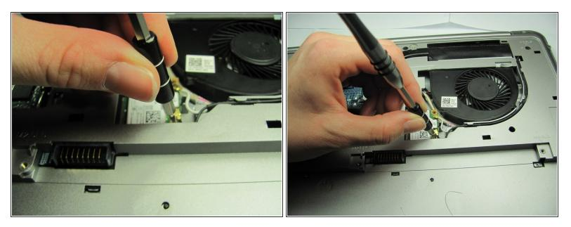
Completely unscrew the 2 mm screw that connects the WiFi card to the mother board using a Philips head screwdriver.
