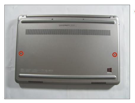
Remove the two 5 mm interior screws that connect the cover to the assembly using the same Philips head screwdriver from the previous step.
