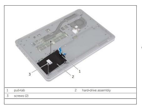
The model device did not come with a hard drive. However, you will need to remove the hard drive to proceed.
