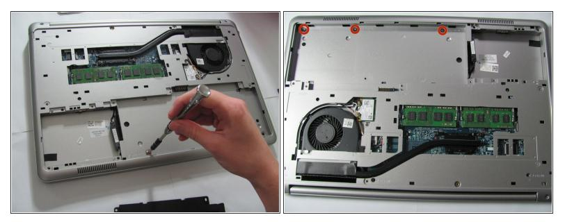
Remove the three silver 2 mm screws (with large flat circular heads) from where the battery was taken out with the Phillips head screwdriver.
