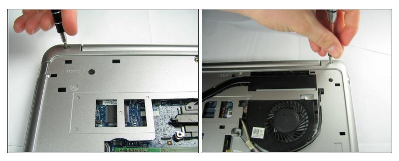
Flip the computer and remove the two silver 5 mm screws on the corners of the base cover with the Phillips head screwdriver.
