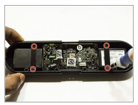
Remove the four 6 mm screws holding the band in place using a Phillips #0 screwdriver.
