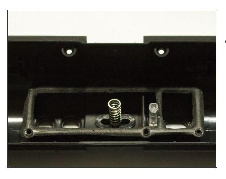
Remove the power button and springs.
