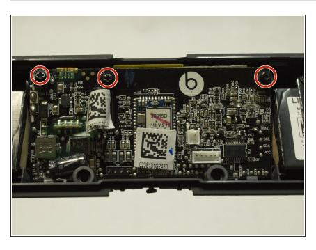
Remove the three 9 mm screws from motherboard and rubber stopper using a Phillips #0 screwdriver.
