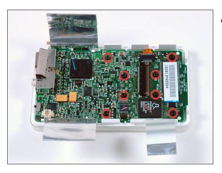
Remove the 8 T6 Torx screws from the logic board.
