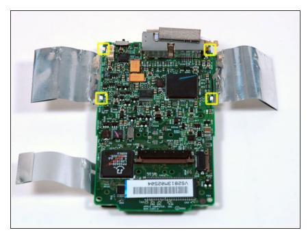
Note the location of the four white plastic tabs securing the display to the logic board. These tabs must be released before the display can be removed.
