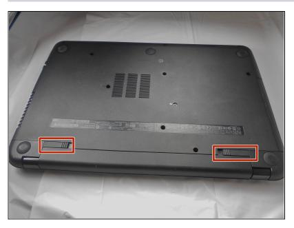
There are two battery release switches circled.
