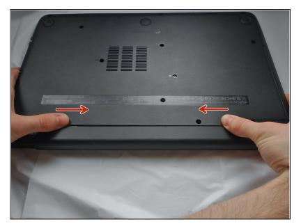
slide release switches inward towards each other to release battery.
