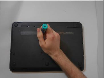
There is one screw holding the DVD±RW Drive in place. Use the #00 screwdriver to remove the screw.
