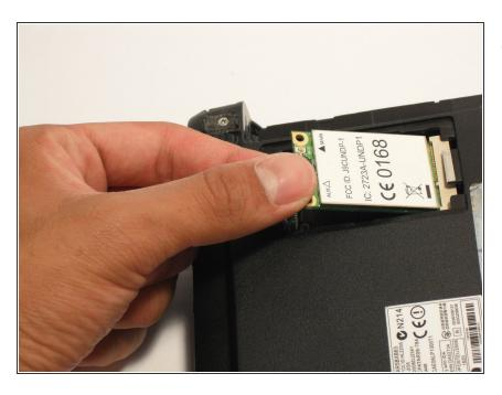
Gently lift up the left side of the wireless card and slide the card out of its socket.
