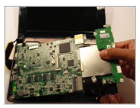
Lift the entire motherboard assembly out the case.
