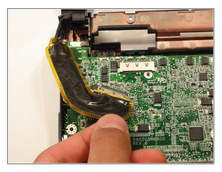
Disconnect the display cable from the top left of the motherboard.
