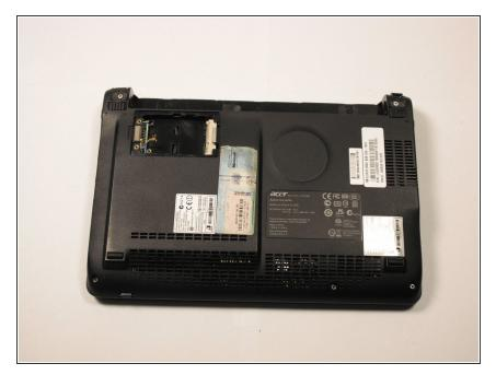
Close the display and turn the ZG5 over so that the battery compartment faces away from you.
