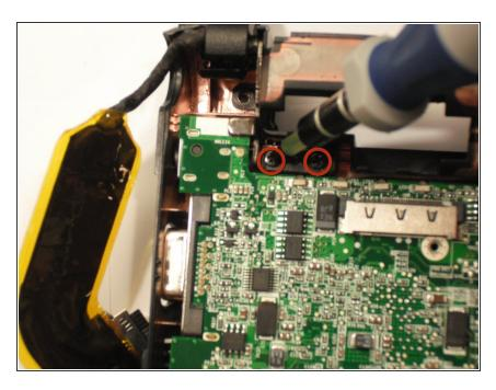
Remove the two 4.7 mm Phillips #1 screws that connect the display to the motherboard.
