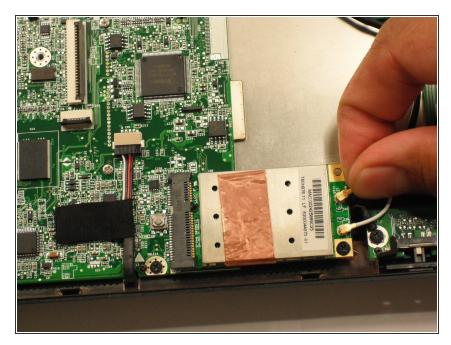
Disconnect the two antenna cables from the right side of the wireless card.
