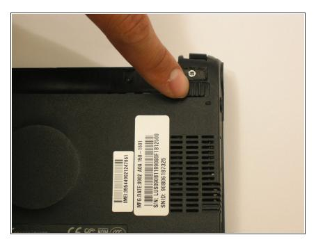
Slide the latch located on the opposite hinge from the lock while pushing the battery up.
