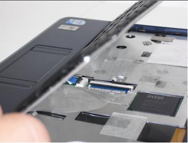
• Lift top of keyboard up. If it doesn't lift easily, there may be tabs on the sides - use the tool to ease them aside and/or shift the keyboard from side to side.
