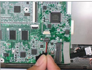
Disconnect the speaker cable from its socket on the motherboard.
