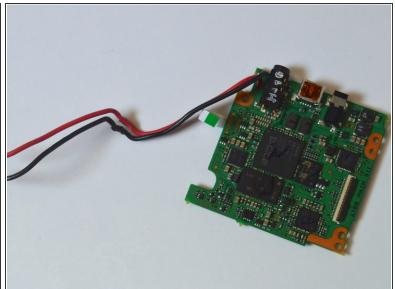
Use the soldering iron to melt the wire contact points and detach the motherboard.
