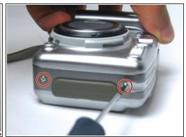
Remove the six 4 mm screws on the sides and bottom of the camera using a Phillips #00 screwdriver.
