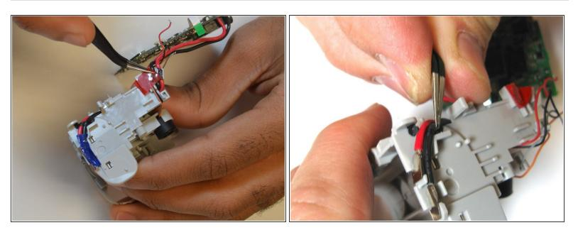
Use the tweezers to remove the red tape and rubber strap to begin removing the wires from the plastic hooks.
