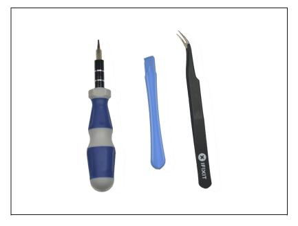
• You will need a Torx T5 screwdriver, plastic opening tool, and a pincet for this operation. Step 2
