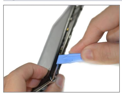
Place the plastic opening tool in-between the black external case of the phone and the silver case, then move it along the edges of the phone to detach the plates.
