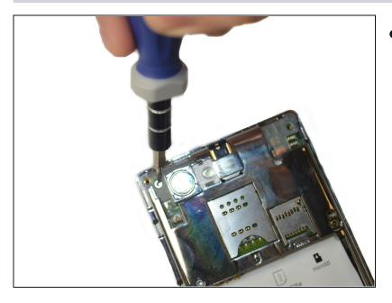
• After removing the top left black plate, you will find another 3.13mm screw. Just remove it by using the screwdriver.
