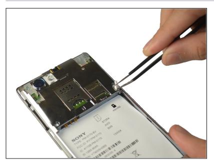
Remove the silicone cover by squeezing it with the <u>tweezers</u>, there is not much pressure needed.
