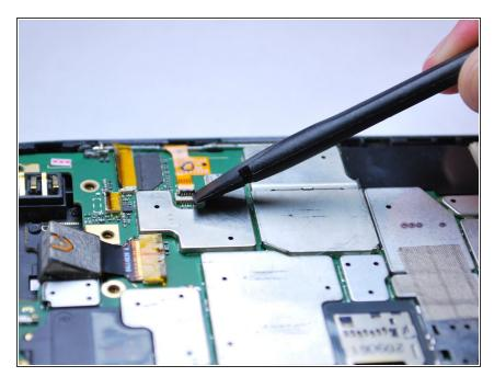
Release the yellow flex cable on the right side of the phone using the spudger by lifting up on the retaining clip.
