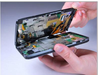
Gently push the screen toward the top edge of the phone and tilt the screen to reveal the black flex cables.
