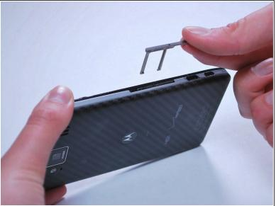
• To remove the SIM card, use an unfolded paperclip to press down on the metal plate on the left side of the phone until it pops up.
