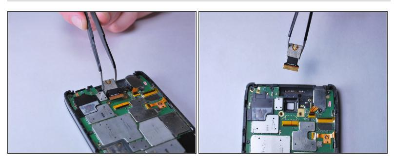
Use tweezers to gently remove the rear-facing camera by lifting it up off of the motherboard.
