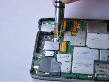
Using a T5 Torx screwdriver, unscrew the two 4.0mm screws on the rear-facing camera cover.
