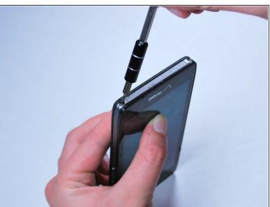
Use the Torx T5 Screwdriver to remove two 5.0 mm screws at the bottom of the phone.
