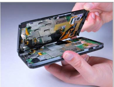
Gently push the screen toward the top edge of the phone and tilt the screen to reveal the black flex cables.
