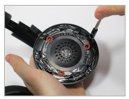
Remove three 7 mm Phillips #00 screws holding the speaker in place.
