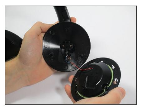
Carefully open the back casing, exposing the speaker wires.
