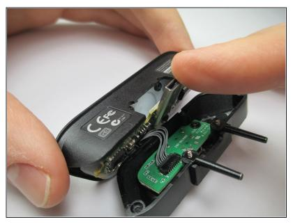
Pull back on the controller USB connector with your finger to separate the main adapter circuit board from the rubber mold in the button panel.
