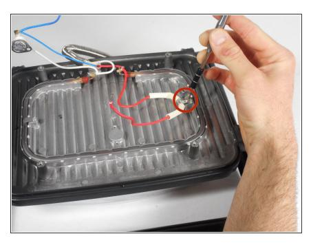
Using the PH2 screwdriver, remove the single 10mm screw connecting the red wiring cover to the cooking surface.
