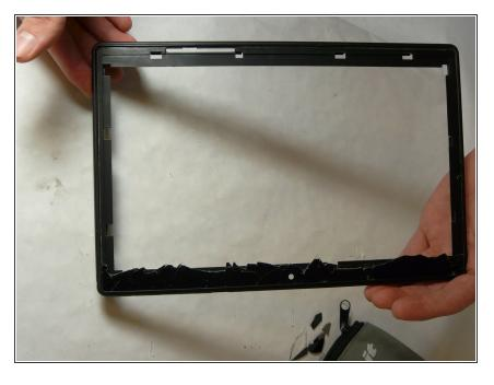
Carefully remove glass. If glass is already broken use gloves to remove glass.
