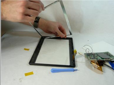
Using the plastic pry tool remove metal frame.
