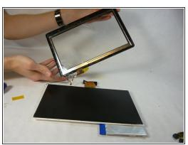
Using a plastic opening tool, remove the back screen pieces from the back.
