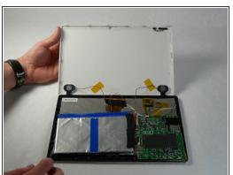
Remove back case of tablet by taking spudger tool to lift the back plate.
