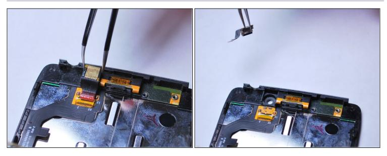
• Use <u>tweezers</u> to remove the front-facing camera by lifting it from the LCD display frame.
