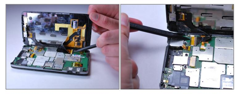
• Release the two black ribbon flex cables by gently pulling up on the connection using the spudger. Then lift the screen to remove.
