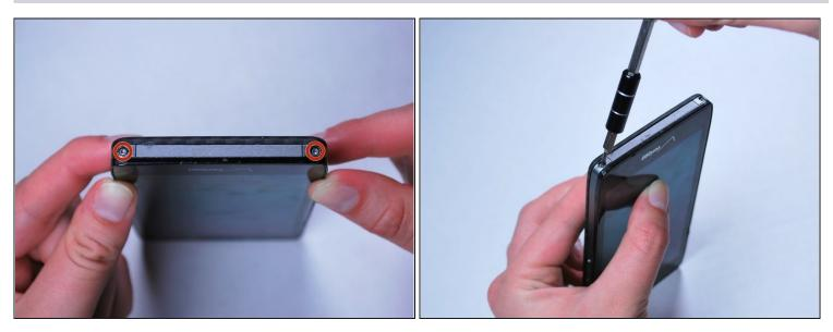
• Use the Torx T5 Screwdriver to remove two 5.0 mm screws at the bottom of the phone.
