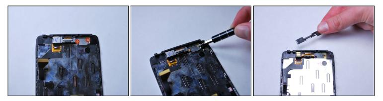
• With a Torx T3 screwdriver, unscrew the two 2.0 mm screws on front-facing camera mounting bracket. Then lift to remove it.
