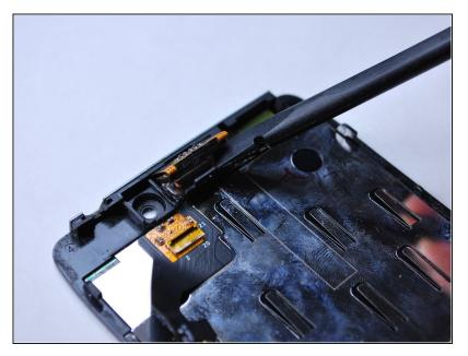
• Insert the spudger between the speaker and retaining clip and gently pry upward to release the earpiece speaker.
