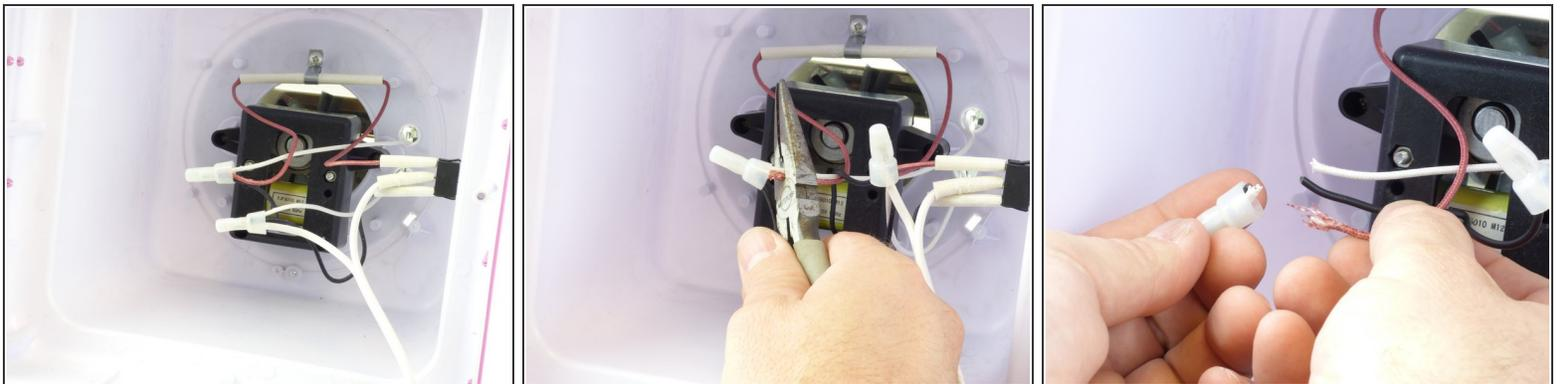
⚠ Make note of the wiring arrangement of each bundle before this step.
