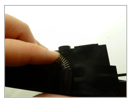
Use your fingernail to squeeze down on one side of the spring and reposition the spring back on to the plastic nipple attached to the smaller part of the game cartridge frame.
