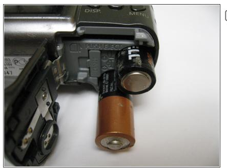
When replacing the AA batteries, verify they are oriented correctly by following the (+) and (-) signs on the camera.
