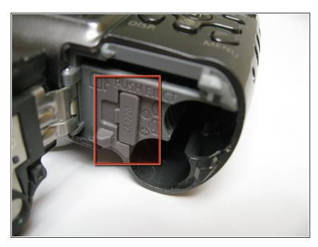
• To access the clock battery, find the clock battery cover, shown here in the red square.
