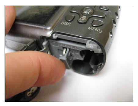
• When accessing the clock battery, use a fingernail or similar small instrument to gently pull the tab out.
