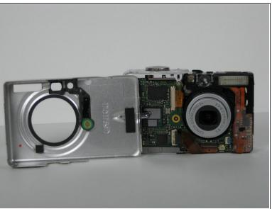
Use your fingers to carefully pry off the front casing of the camera. The front casing should pull straight off.
