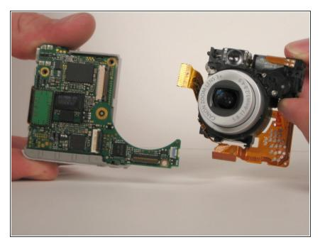
Pull the lens assembly away from the motherboard assembly.
