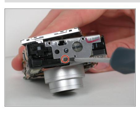
Remove the one 2.7 mm Phillips screw from the left side of the camera.
