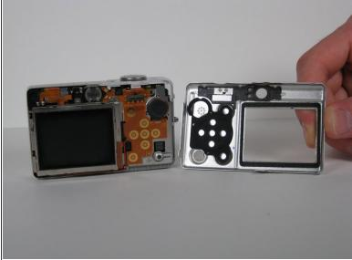
Use your fingers to carefully pry off the back casing from the camera assembly.
