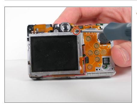
Remove the one 2.4 mm Phillips screw directly above the top right corner of the LCD screen.
