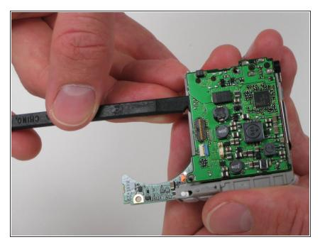
Use the flat end of the spudger to loosen the connection from the battery holder and gently pry the side of the motherboard off of the battery holder.
