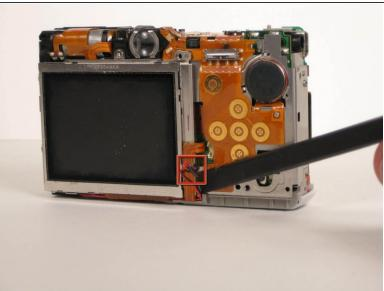
Use the flat end of the spudger to lift up the small black connector from the back side of the motherboard. The connector should just lift straight up.
