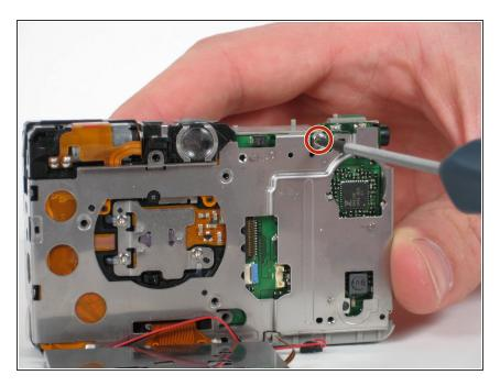
Remove the one 4.3 mm Phillips screw that is now visible, which is located at the top right of the back of the camera.
