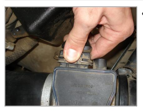
Reattach the electronic cable to the MAF.
