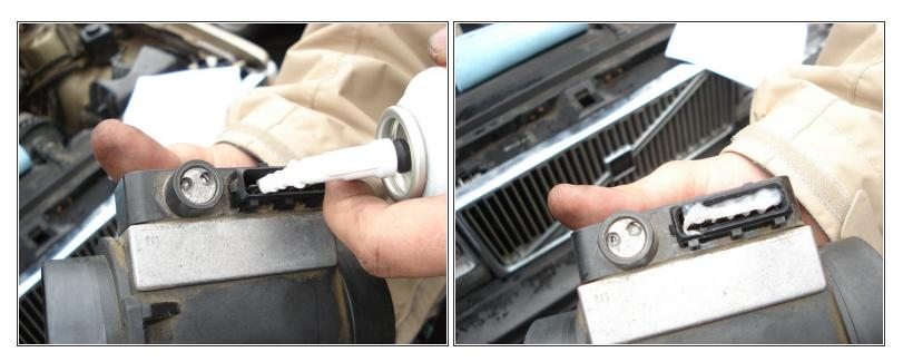
• Inject conducting lubricant into the MAF sensor electronic coupling.
