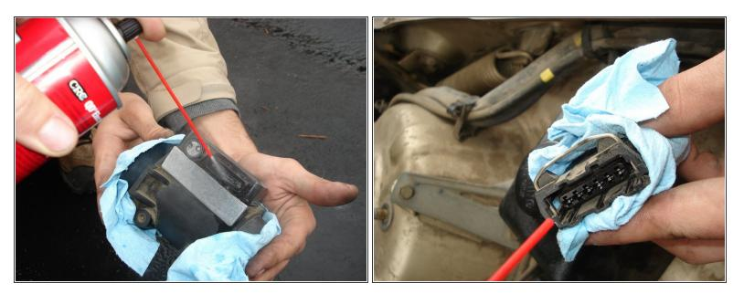
• Clean the electronic coupling with an electronics cleaner.
