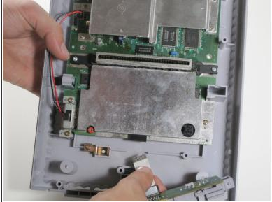
Carefully remove the ribbon cable from its port.
