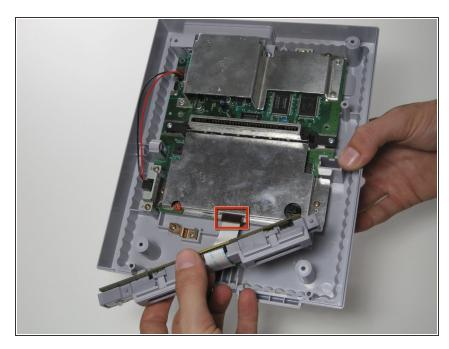
Lift the controller ports out of the housing, this should be done without much force. Take note of the location of the ribbon cable connection.
