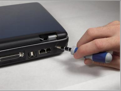
Remove two 8.6 mm screws on the back corners of the laptop.
