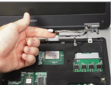
Use the plastic opening tool to remove the wire.
