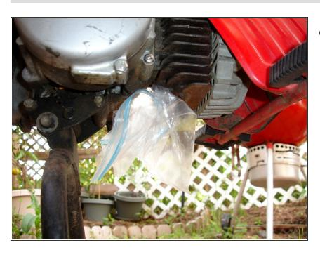
Cover the engine exhaust hole with a plastic bag to keep excess debris from making its way into the engine block.
