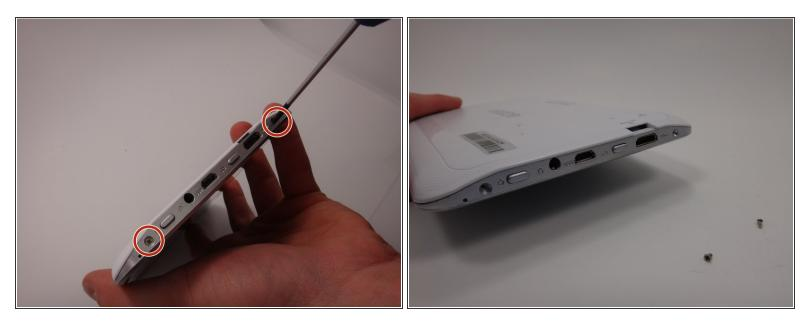
Use a Phillips #00 screwdriver to remove the two 4mm screws found on the top edge of the tablet near the power button.
