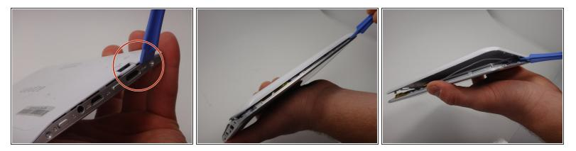
Use the plastic opening tool to pry the white back from the silver frame. Start near the micro SD slot.
