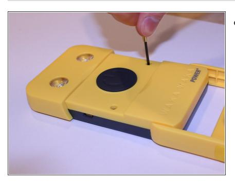
Remove the two 5mm screws with a #0 Phillips screwdriver.
