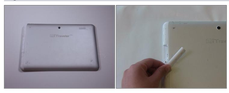
• With the device face down, slide the charging port cover off on the left side of device.
