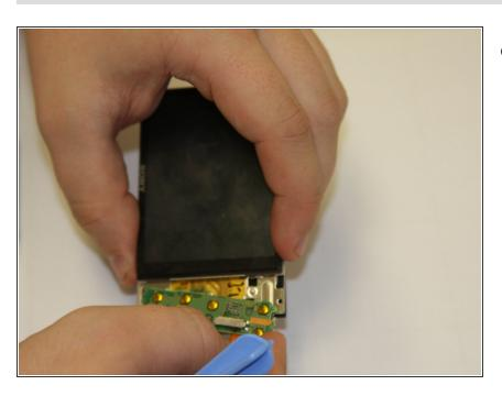
Remove and replace the button circuit board.
