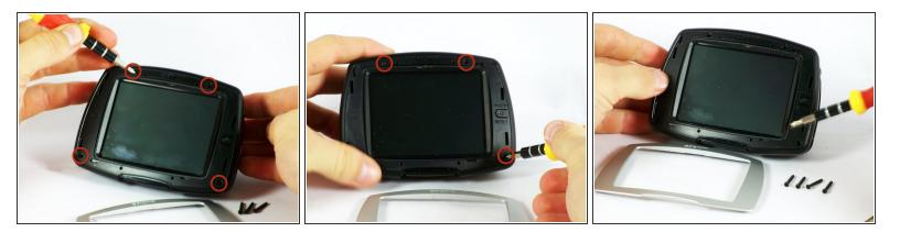
• Use a Phillips #00 screwdriver to remove the four screws around the screen.
