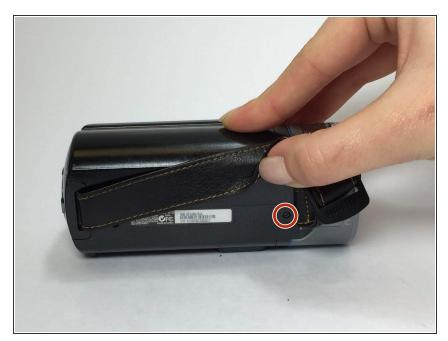
• Remove the 4 mm screw next to the buckle of the hand strap closest to the lens.
