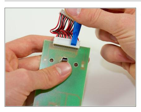
Using a plastic opening tool or a similar tool, gently pry the power ribbon cord out of its port.
