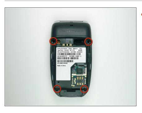
To remove the back case first remove the four screws shown with a T5 Torx screwdriver
