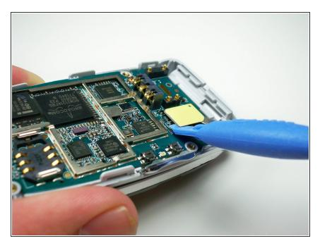
Flip up the yellow tab using a plastic opening tool to disconnect the motherboard from the phone body.
