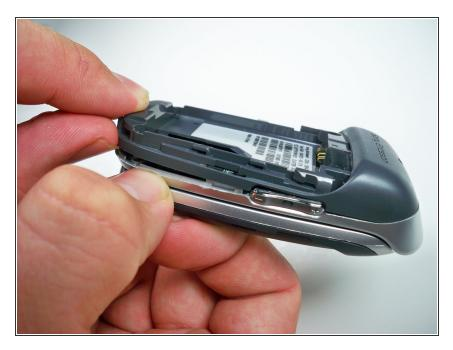
Using your fingernail lift up the side of the casing around the bottom of the phone to release all five of the clips.
