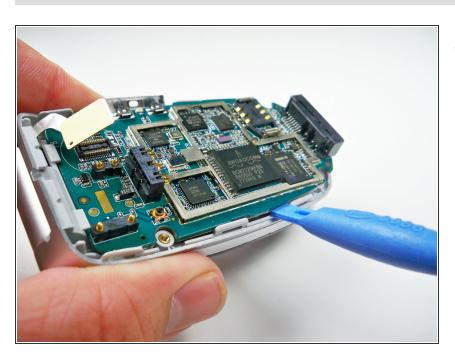
Work the plastic opening tool around the edges of the motherboard to release it from the clips.
