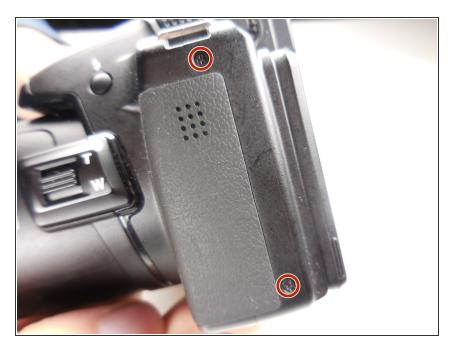
On the opposite side of the camera, remove the two 3mm PH00 Philips screws.
