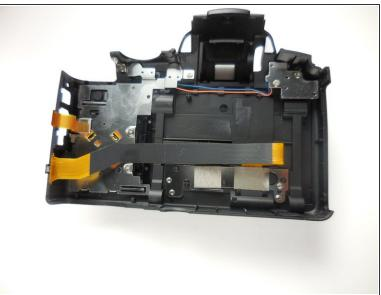
Unplug the two ribbon cables to completely detach the back.
