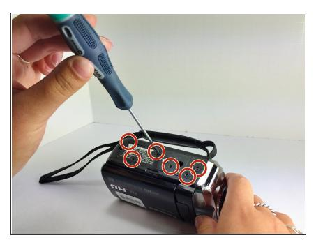
Next, unscrew the six .5 mm Phillips #00 screws on the bottom of the camcorder.
