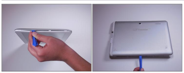
• Move around the device with the plastic opening tool, pushing down to release the back plate from clips.
