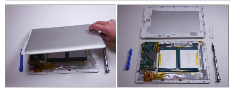
• Once you've moved around the whole device with the plastic opening tool, the back plate will completely release from the rest of the device.
