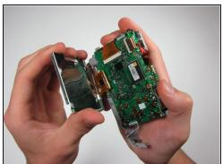
Gently grab the sides of the LCD casing and remove it from the camera
