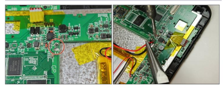
• Solder the red battery wire to the point labeled BATT +, and the black battery wire to the point BATT -.
