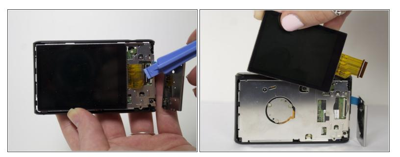
Remove the yellow cable by pulling gently upwards, away from the inside of the camera, until it separates from its port.
