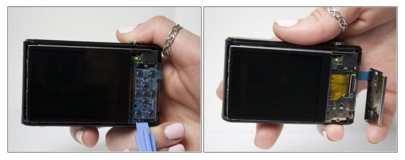
• Separate the button panel to reveal the port holding the screen on.
