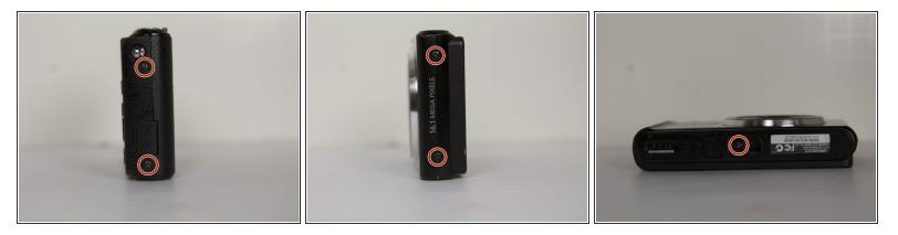
• Use a Phillips head screwdriver to remove 5 screws from the camera. There are 2 4mm screws on the left side, 2 2mm screws on the right side and 1 4mm screw on the bottom.
