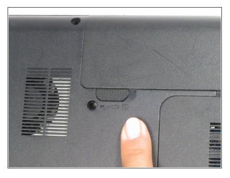
Release the locking mechanism by switching the left slider to the left.
