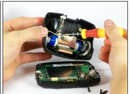
Use a Phillips #00 screwdriver to remove the two screws from the battery bracket.
